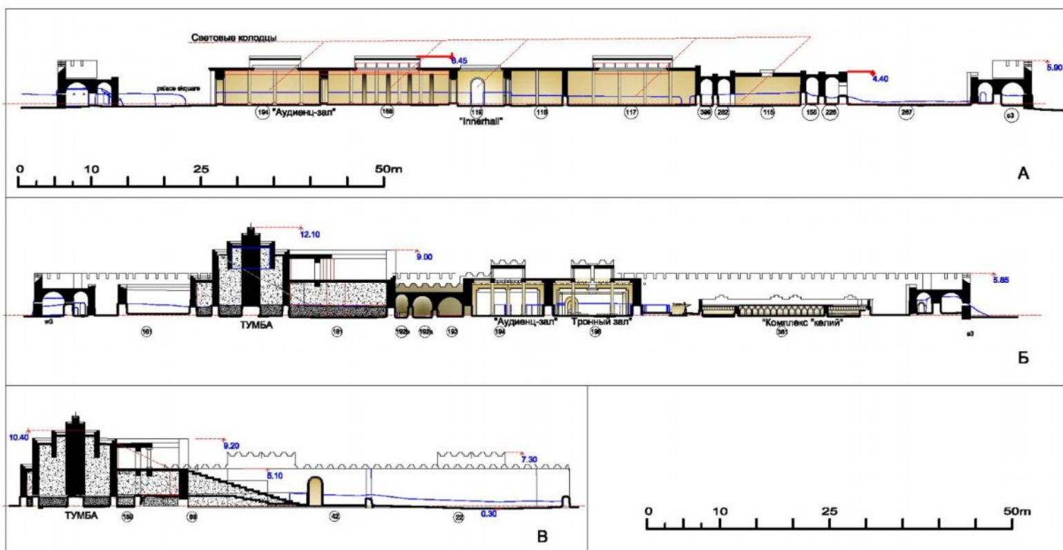
25. Palace. The scheme of reconstruction of buildings. Cross-sections 1-1, 2-2, 3-3. A – north-south cross-section 1-1. Б – west-east cross-section 2-2. B – north-south cross-section 3-3 along the "Sand Rooms (North Complex)".
